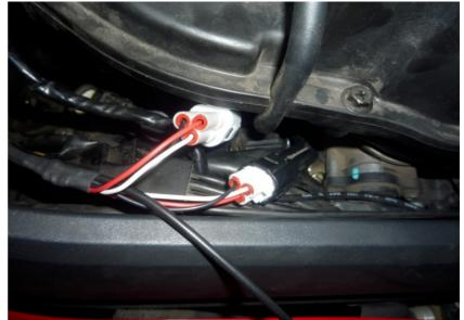
Connect the GPX Black/Green wire to the Blue/Purple wire of the crankshaft position sensor.
