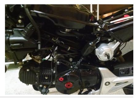
Locate the speed sensor connectors in the dust boot and disconnect it.
