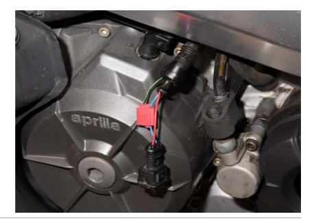
Connect the GPX Red wire to the Green wire of the rear brake light switch connector.
