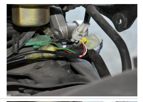
Connect GPAT G2 Red wire to the Orange wire of the rear brake light switch connector.
