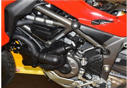
Plug the Gipro connectors in-line with the gear position sensor connectors.
