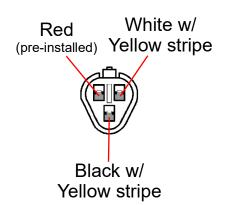
**8.** Insert the two male terminals into the **larger** 3-pole plug adapter through the back until they click into place.
