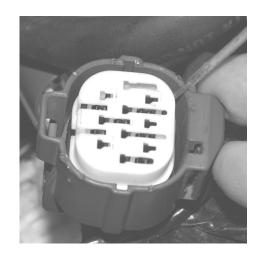
**6.** Release and remove the MIDDLE two terminals from BOTH plugs.
