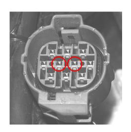
**7.** Insert the two female terminals into the **smaller** 3-pole plug adapter supplied through the back until they click into place.
